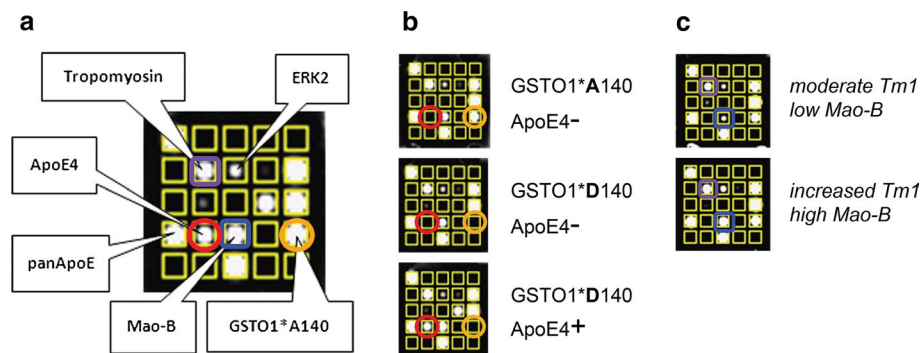
Fig. 2 Schematic representation of the new AD multiplex protein biochip. a Antibodies directed against the proteins of interest were spotted on the biochip, incubated with samples (or calibrators) and target analyte concentrations quantified by measuring chemiluminescence signals of bound HRP-labelled secondary antibodies. b Quantification of GSTO1*A140 (orange circles) and ApoE4 (red circles)
