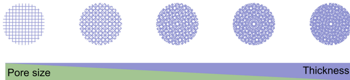
Fig. 1 Schematic illustration describing the pore structure evolution during the separator manufacturing process. It can be seen that thin separators exhibit larger pores and a higher porosity than thicker separators composed of more cellulose fibers
