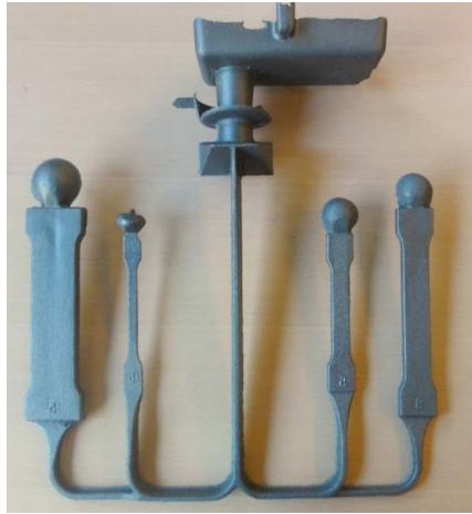
Fig. 21. The lay-out of casting specimens [Moumeni, Tutum, Tiedje and Hattel, Paper I]
