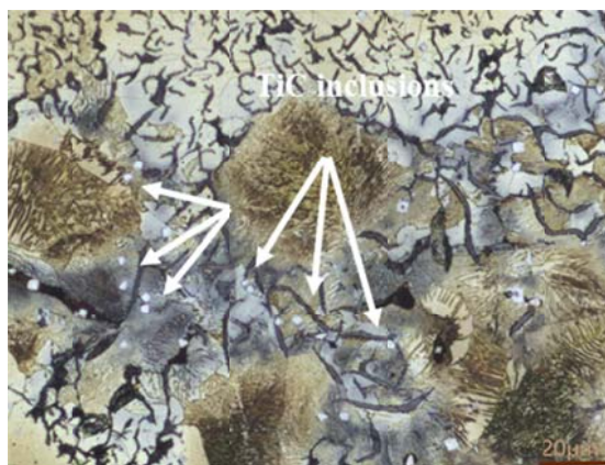
Fig. 44- Colour etched sample GI.3; TiC inclusions indicated [Moumeni; Tiedje and Hattel, Paper II]
