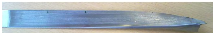
Figure 5.50: Broken strip from SRT2.
