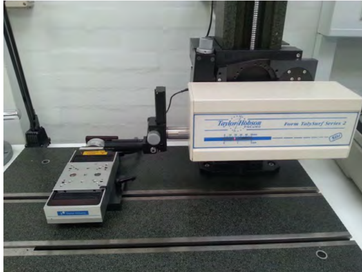
Figure 2.33: Form TalySurf 50 Inductive.
