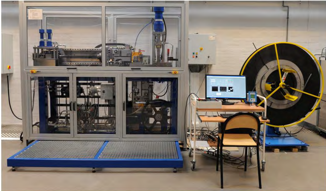
Figure 5.5: New universal sheet tribo-tester present in DTU tribo-laboratory [157].
