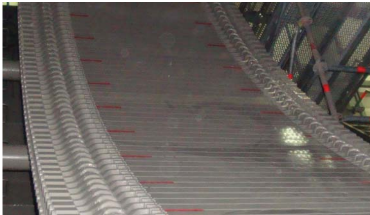
(b) Section of stator with windings
