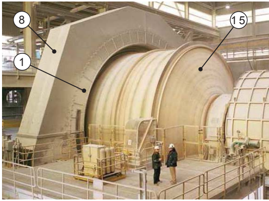
(a) SAG mill with a gearless drive
