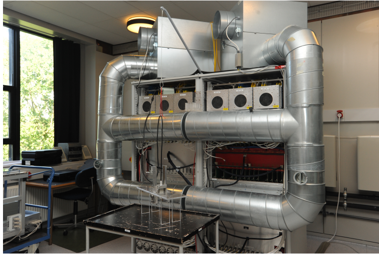
Figure 5.8 A photograph of SARUS, which has 1024 channels distributed over six transducer plugs. The phased array transducer used for the measurements in this chapter has only 128 elements. Therefore, it is plugged to one of the six sockets. The transducer is positioned in the transducer fixation device, which can be placed in the flow-rig water tank. Photo courtesy of Morten Fischer Rasmussen.
