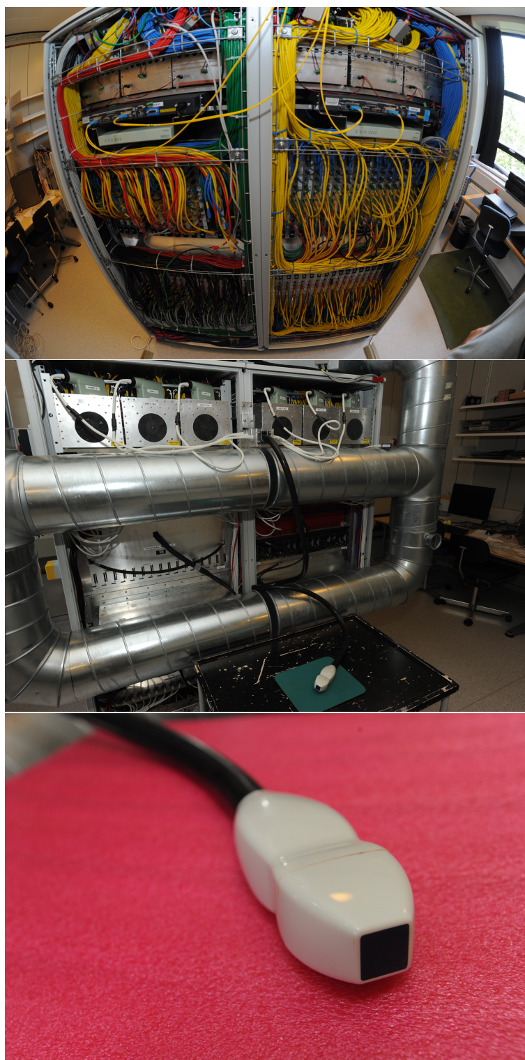
Figure 7.1 Photographs of (from top to bottom) the back of SARUS and the many cables needed for sampling from the 1024 channels, the front of SARUS with the six transducer plugs required for the 2D transducer connected, and a close-up of the 2D transducer. Photos courtesy of Morten Fischer Rasmussen.
