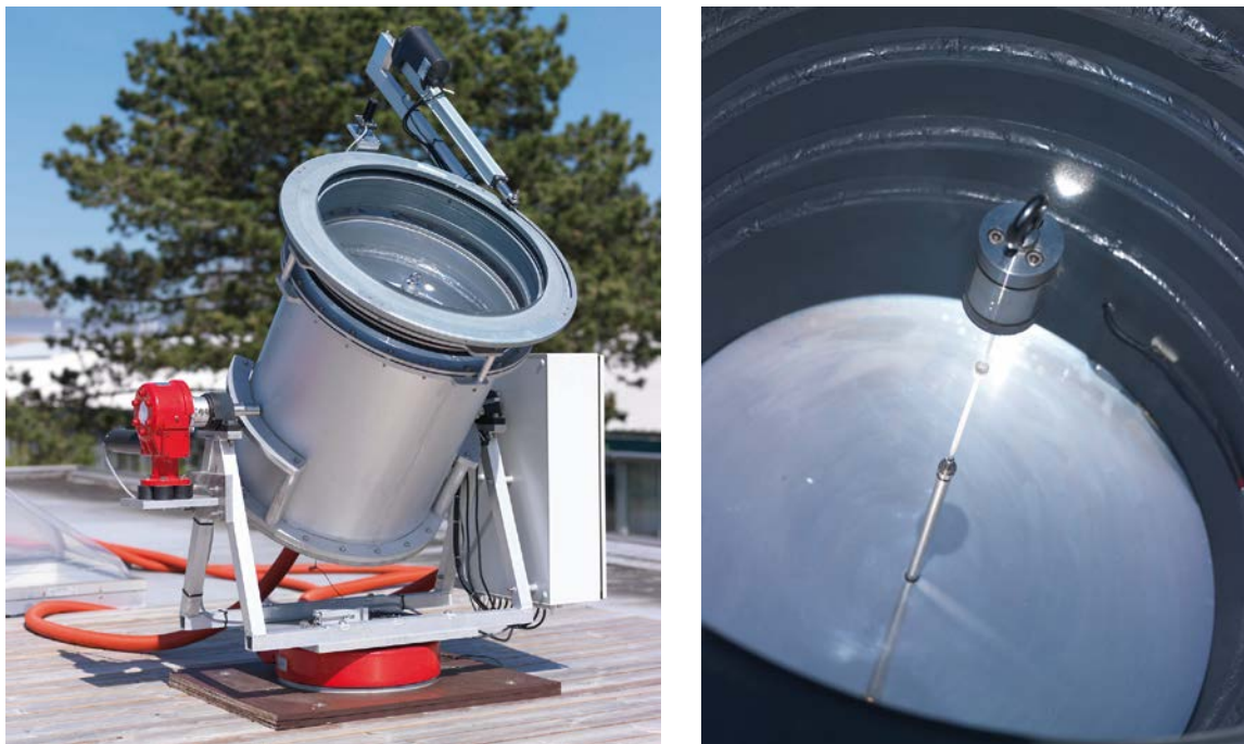
Figure 4.10. Solar concentrator (left) and close-up of fiber (right).
