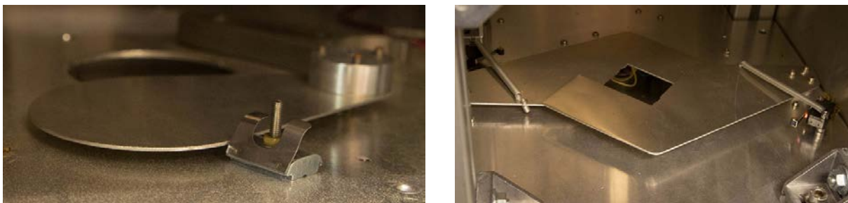
Figure 4.2. The iris (right) is an aluminum plate, moved by a stepper motor with a gear reduction. The shutter plate (left) is operated by a rotary solenoid.
