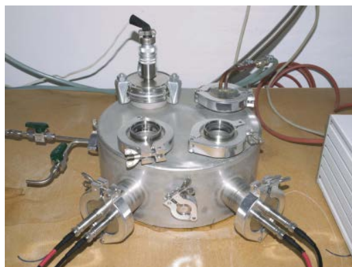
Figure 5.3. Atmosphere chamber used for controlled atmosphere degradation.
