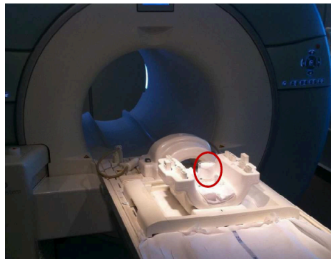
Figure 5.9: One of the heel pad model (marked by the red circle) placed at the entrance of the MRI scanner
