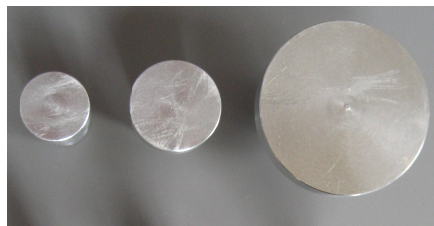
Figure 4.2: The three different pistons used for the compression test. From the left, diameter of 15, 20 and 40 mm.
