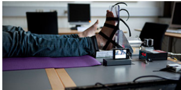
Figure 3.6: Location of the compression device and its equipment. The volunteer lies in a supine position with both legs straight and relaxed.
