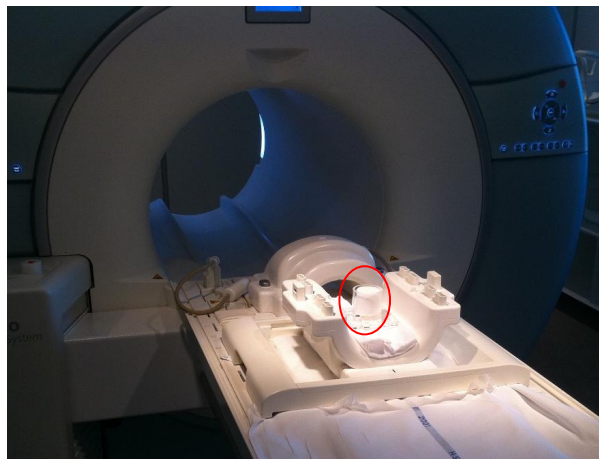
Fig.4 Heel pad phantom (marked by the red circle) placed inside the coil in the MRI scanner
