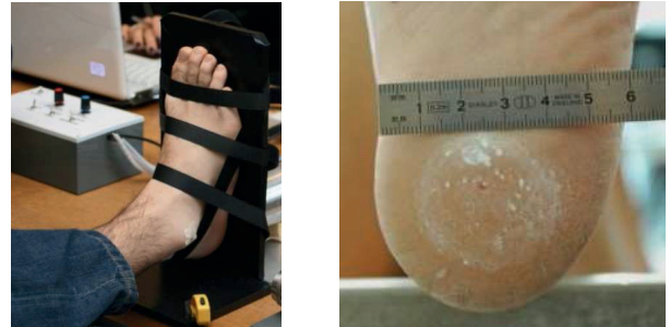
Fig. 2 Position of the foot on the vertical plate, on the left. Position of the cylinder on the heel pad, on the right. The print of the cylinder is made by placing some talcum powder on its surface
