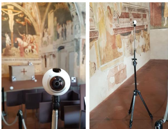
Figure 6. Image acquisition can be carried out by placing the camera on a tripod; the camera can be pointed to any direction.
