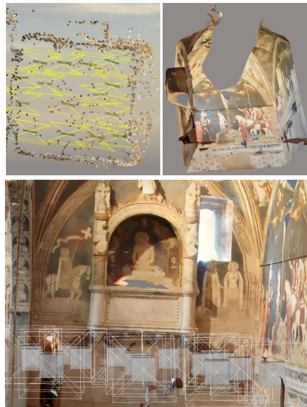
Figure 9. The reconstruction from front rear facing fisheye images has a better accuracy but is partially incomplete, especially the area above the camera.
