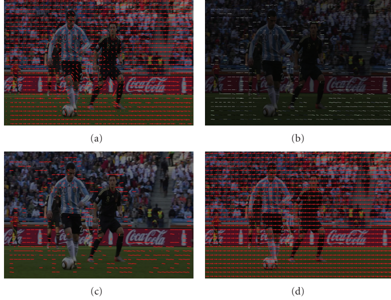
FIGURE 1: Reliable motion information extraction. (a) all motion vectors; (b) motion vectors reliability; (c) reliable motion vectors; (d) estimated camera motion.
