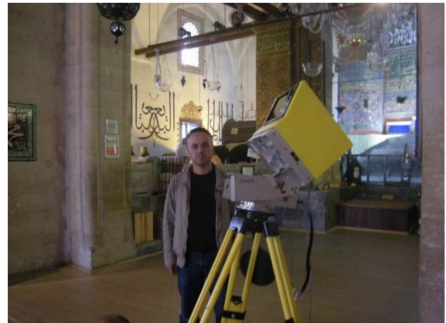
Figure 2. Laser scanning in Huzur-ı Pir section of Mevlana Museum.
