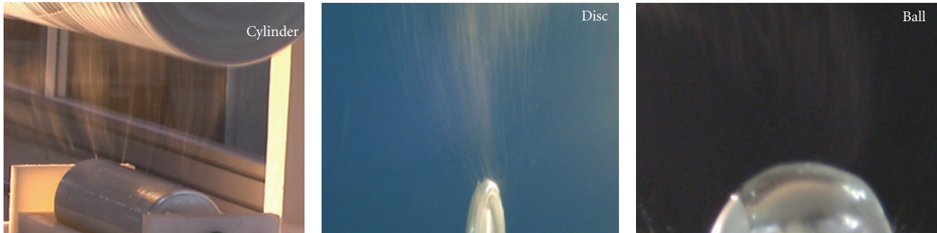
FIGURE 5: Photographs of cylinder, disc and ball electrospinning processes (Cylinder diameter 80 mm, rim radius 5 mm; ball diameter 80 mm; disc diameter 80 mm, thickness 2 mm) [45].
