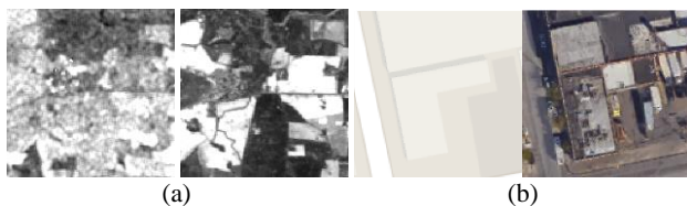
Figure 1 Example of different intensity and texture patterns between multimodal remote sensing images. (a) SAR (left) and visible (right) images. (b) Map (left) and visible (right) images.
