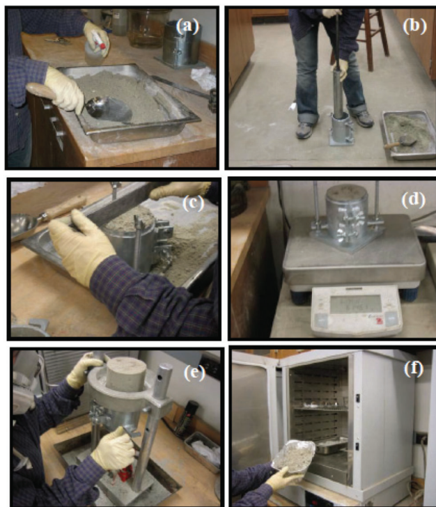
Figure 2.5 Compaction procedure for in situ soil, soil-steel slag-Class-C fly ash mixtures and soil-steel slag-blast-furnace-slag mixtures: (a) spraying water to achieve the desired water content, (b) compacting the sample in a 4-inch-diameter mold, (c) trimming the compacted sample, (d) measuring the compacted mass, (e) recovering the sample with a hydraulic jack, and (f) oven drying for water content measurement.
