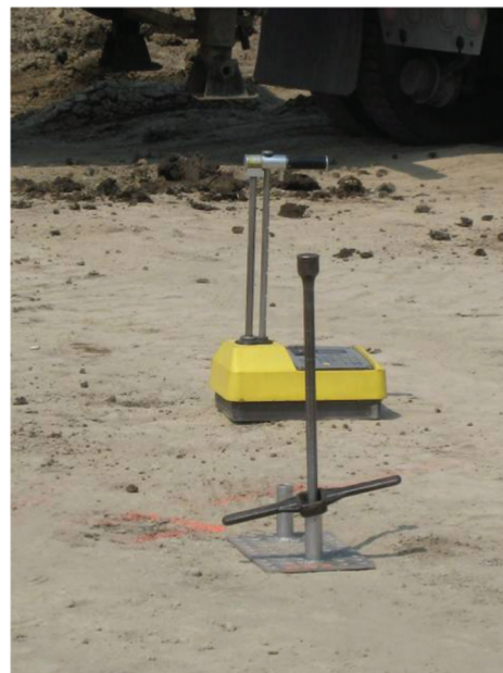
Figure 4.10 Nuclear gauge measurements on subgrade soils stabilized with 7% steel slag-3% Class-C fly ash mixture.
