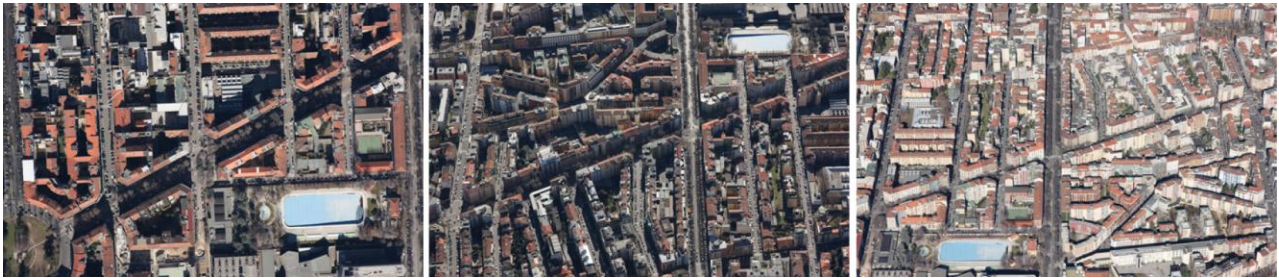
Figure 2: Same urban scene, acquired with a Midas 5 system, viewed from different perspectives (nadir and two oblique, respectively).
