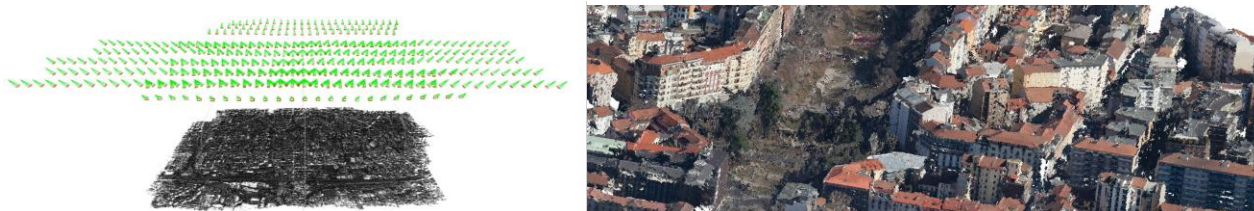
Figure 1: Large urban area pictured with an oblique multi-camera system. Once advanced image triangulation methods have retrieved interior and exterior parameters of the cameras, dense point clouds can be derived for 3D city modelling, feature extraction and mapping purposes.
