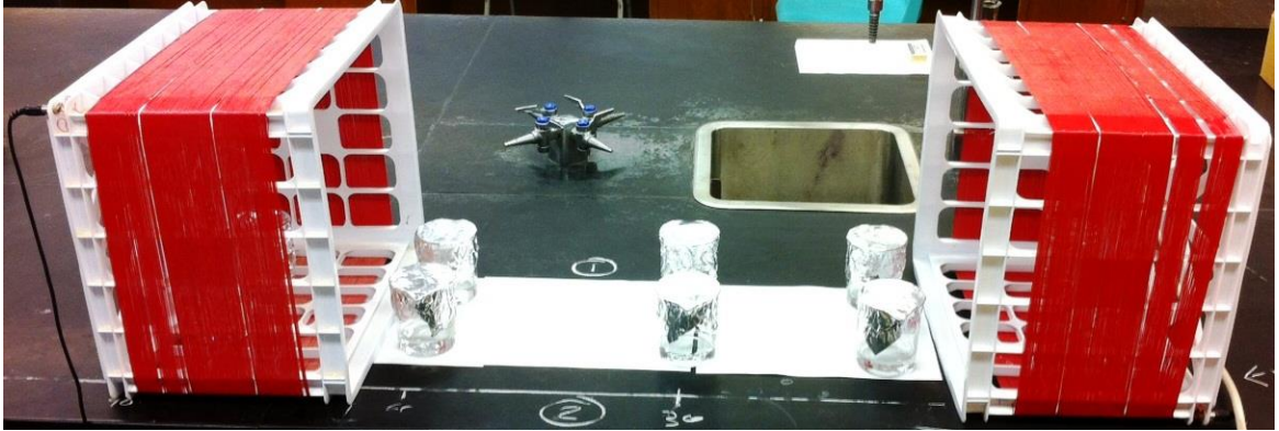
Figure 1. The experimental equipment. When one of the two coils was activated, the proximal containers were location A, the middle were middle MA, and the distal is inactive (NA).
