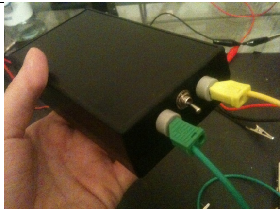
Switch placement between voltage ports
