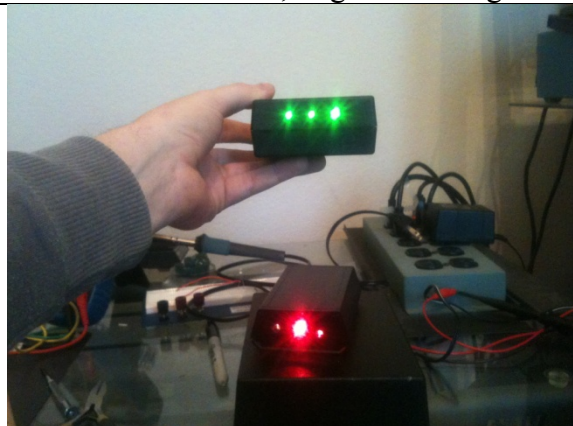
Wireless power transfer through multiple stackable units. Version 1.0 on bottom, version 1.1 held above
