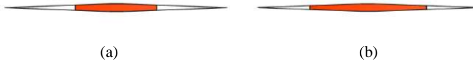
Figure 6.8: Mercury intrusion into a large-aspect-ratio throat which is adopted in the nooks and crannies (NC) model. The non-percolating increase in mercury saturation after an increase in the capillary pressure is to occupy the corners. Compare (a) and (b) in which the mercury is shown with red color.
