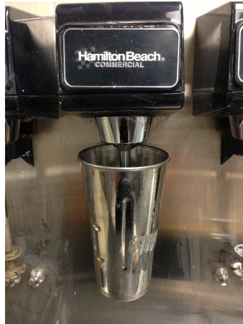
Figure 3-5: Mixing cup with bentonite suspensions on mixer
