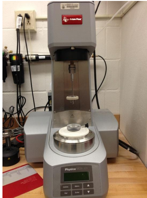
Figure 3-3: Rheometer setup with vane and cup measuring system
