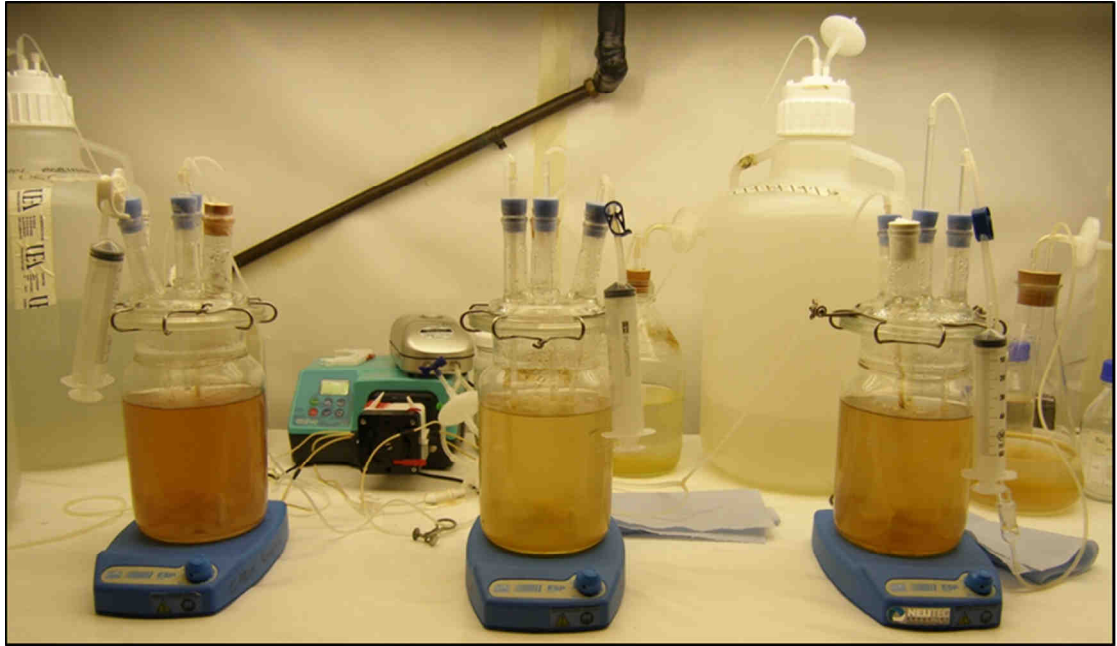
Figure 2.1. Chemostats. From the left; 80:1 N:P ratio culture, 3:1 N:P ratio culture and 16:1 N:P ratio culture.
