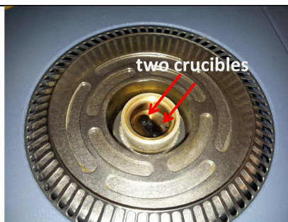
Figure 2.9: Opened furnace with two crucibles in Q-2000 MTDSC.
