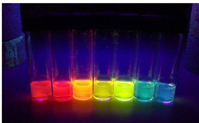
Figure 1.2: The optical properties of Quantum Dots with the absorption profile, full line, and emission profile, dashed line, for an InP@ZnS sample (top) and a photo showing the range of emission colours for InP@ZnS of different sizes synthesised during the course of this work. The size of the Quantum Dots decreases from left to right. A typical InP core diameter is 3.2 nm.
