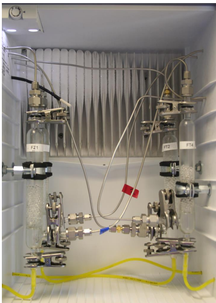
Figure 2.3. Photo of the four glass fridge traps at WAO inside the refrigerator. The stainless steel tubing carries sample air into the base of the fridge traps and it passes up through the glass beads inside the traps and exits through the top of the traps. The yellow tubing connects to peristaltic pump heads that draw off condensed water from the base of the traps. A perforated glass disc just above the sample air inlet prevents the glass beads from blocking the peristaltic drain. In addition, the ball and socket at the sample air inlet have been fused to the trap body at a slight angle, to prevent condensed water accumulating in the inlet tubing instead of the trap itself.
