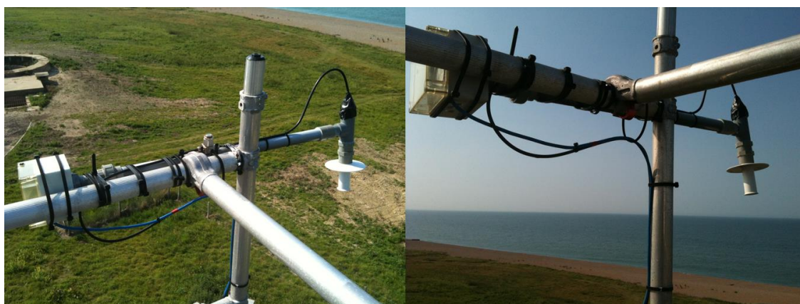
Figure 2.2. Photos of one of the aspirated air inlets fixed to the Weybourne tower.
