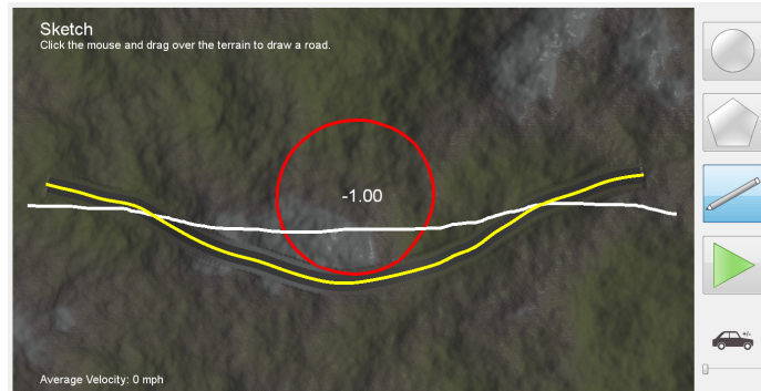
Figure 4.9: The original user-sketch (white) is manipulated in curvature-space so that it avoids the negative ‘Influence Region’ and produces the road in yellow.
