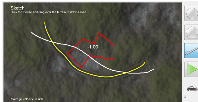
Figure 4.15: The original user-sketch (white) is manipulated in curvature-space so that it avoids the negative ‘Influence Region’, producing the road in yellow.
