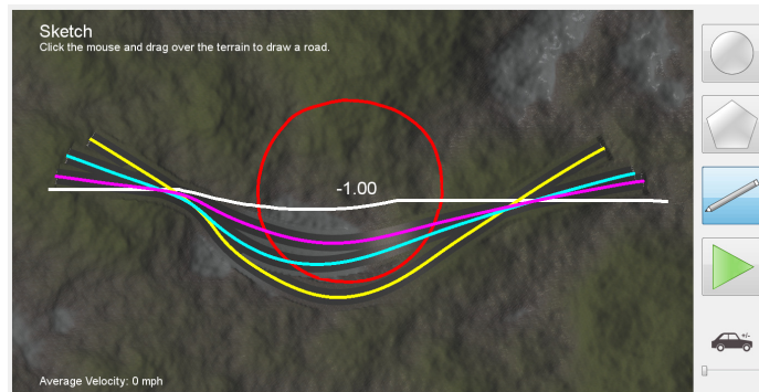
Figure 4.12: Roads with various characteristics can be produced from the same sketch when using different deviation factors. The original user-sketch (white) produces the yellow road when there is no deviation limitation, i.e. when \gamma = 0 , the blue road is produced when \gamma = 0.1 , and the pink road is produced when \gamma = 100 .
