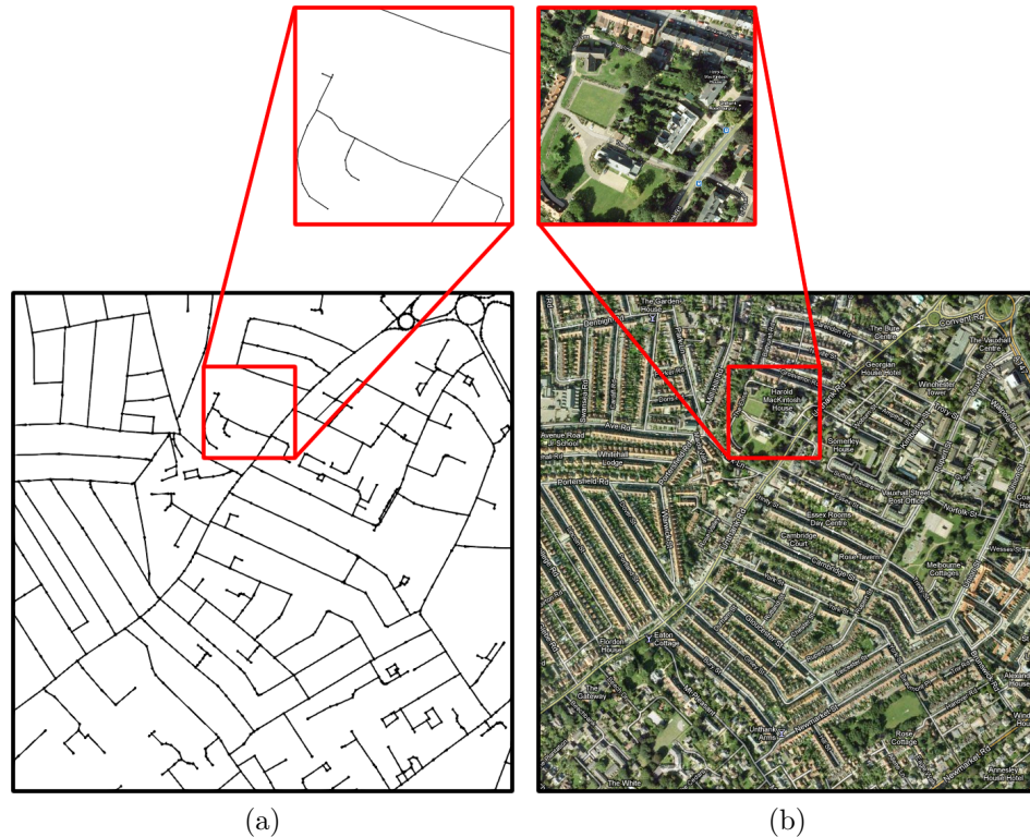
Figure 3.1: (a) Road centre line data for a 1 km 2 tile area of Norwich, United Kingdom. The data is represented as a set of vertices and connecting edges. At the boundaries of the tile there are some isolated edges, created from the tile segmentation. (b) A hybrid satellite image of the same region. There are some discrepancies between the sets of data where mapping information is outdated, as highlighted above. Imagery ©2013 DigitalGlobe, Getmapping Plc, Infoterra Ltd & Bluesky, and The GeoInformation Group. Map data ©2013 Google.
