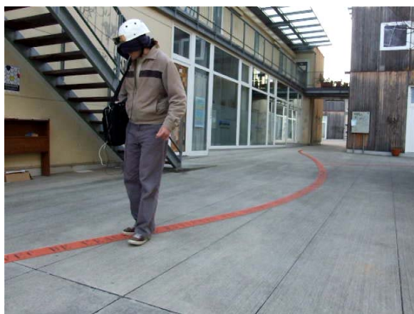
Figure 3. A blindfolded individual following a colored line with a head mounted webcam and a notebook carried in a shoulder pack.
