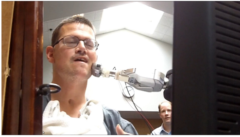
Fig. 12. Robotic Shaving with Force Sensing: Henry Evans shaves himself with a Willow Garage PR2 robot. In this test, the subject was able to obtain nicks and abrasions, motivating the need for intelligent force sensing.
