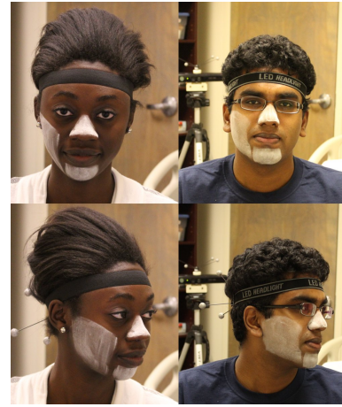
Fig. 5. Talcum powder regions: We applied talcum powder to the cheek, chin, and nose before the wiping trials began.
