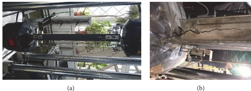
FIGURE 2: Tensile test (a) and zoomed view of LVDT for monitoring slip of the CFRP sheet (b).
