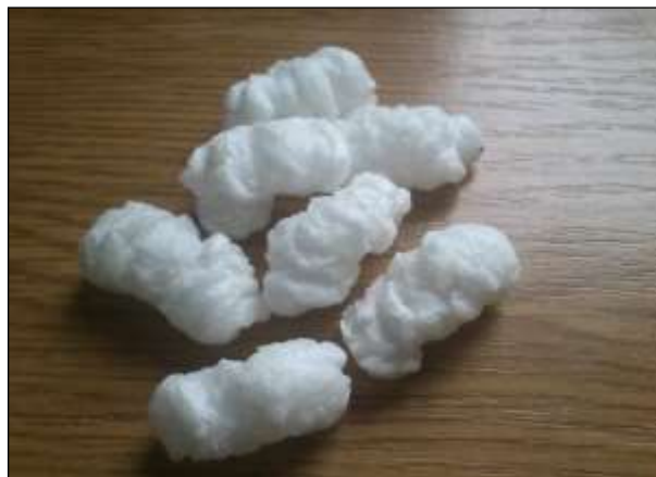
Fig. 5. Starch-based foam materials with Plastronfoam PDE addition.
