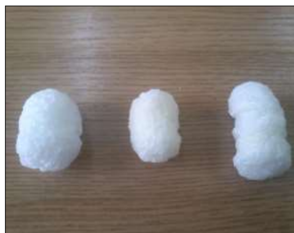
Fig. 7. Foamed starch-based materials with poly(vinyl) alcohol addition, from the left: wheat, corn and potato starch.
