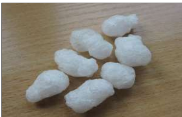
Fig. 6. Starch-based foam materials with poly(vinyl) alcohol addition.
