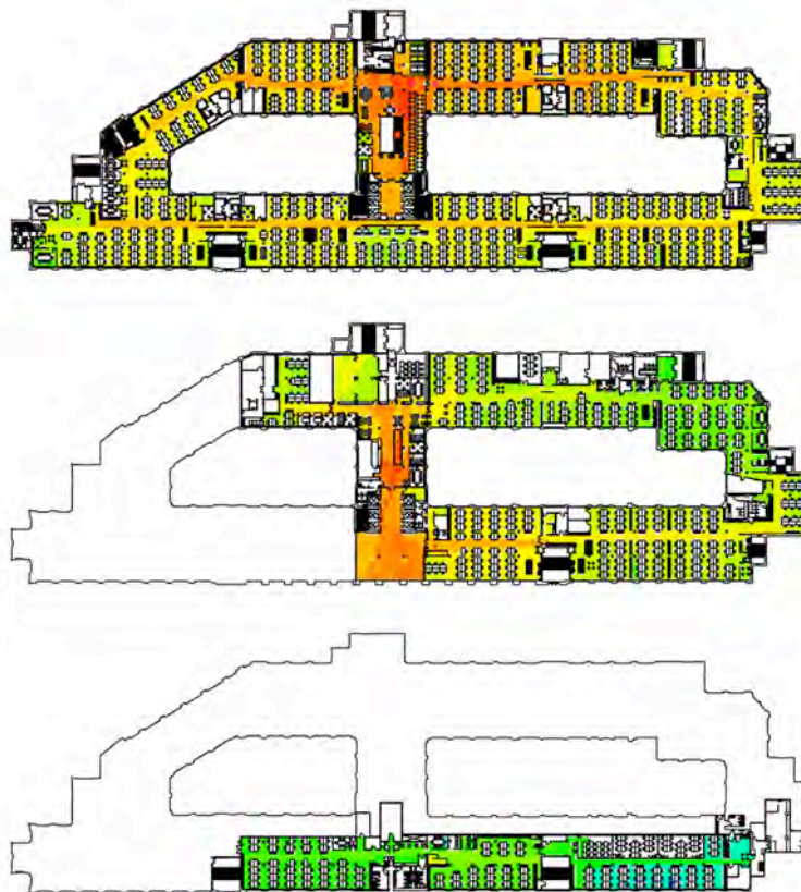
Figure 4: The visual graph analysis (based on accessibility) shows how lobby and café form an integration core, spreading activity and 'buzz' across the large floor plates.
