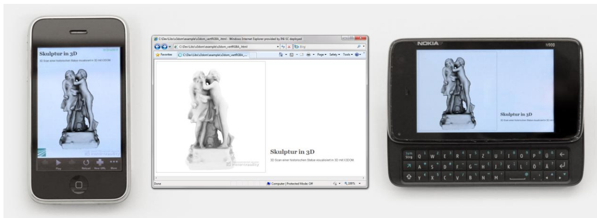
Figure 1. With MeshLab exported model of an old statue visualized via X3DOM in the same HTML page on 3 different platforms: iPhone App using WebKit extensions; Internet Explorer C++ based X3D plugin; WebGL-based implementation on Nokia N900.
