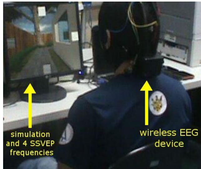
Figure 15. Volunteer using SSVEP to navigate, as using a telepresence robot, in the House Simulation SG. Source: FLORIANO et al., 2016.
