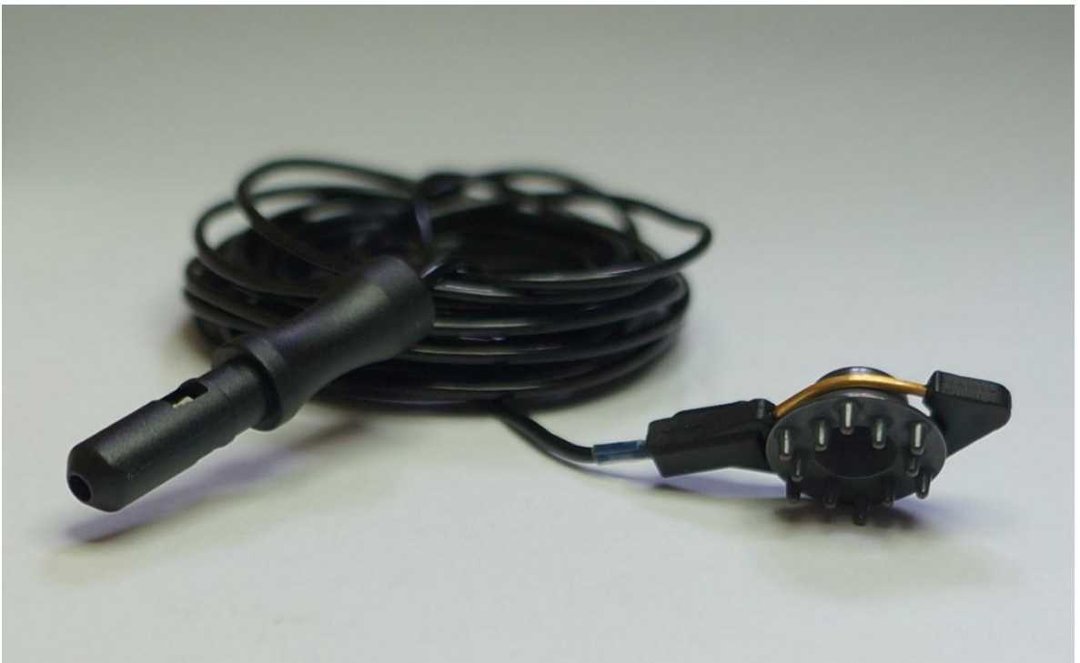
Figure 3. Cable with electrode coupled through a connector at one of its tips, and touchproof connector at its other end.
