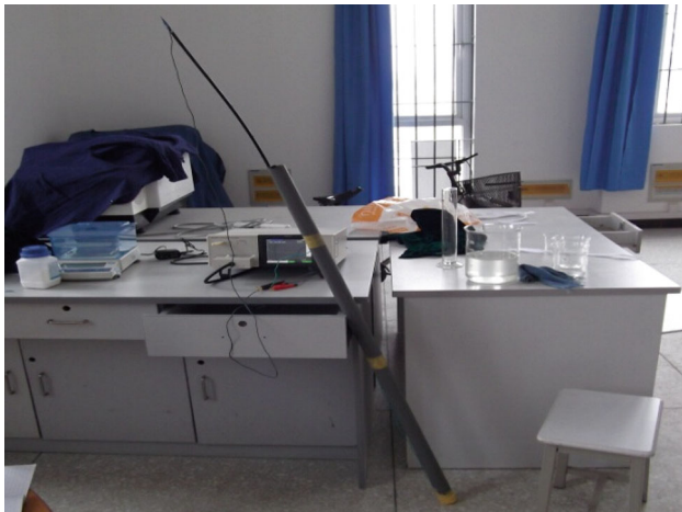
Fig. 7 A PVC pipe with copper wireline and full of NaCl solution, the dimension is length \times diameter = 150 cm \times 2.5 cm
