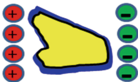
Fig. 5 A single water-wet mineral particle with ions at two sides forming a micro ion capacitor
