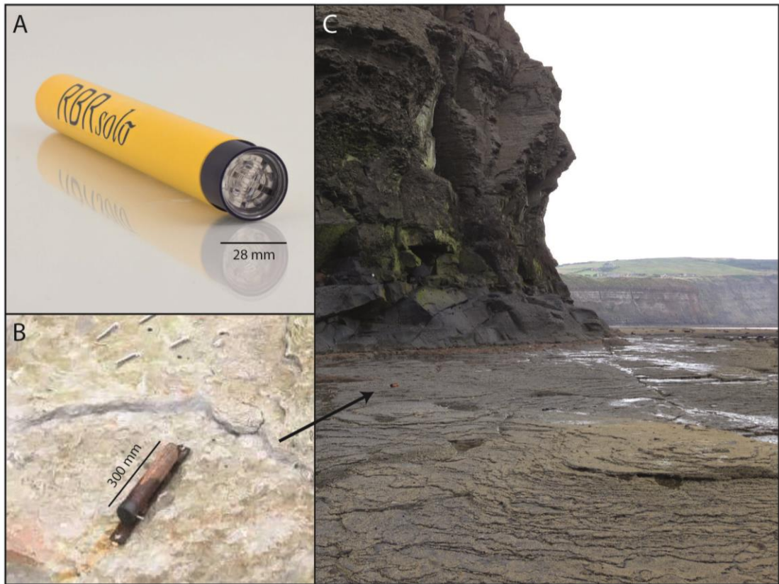
Figure 5.2: A) RBR solo wave gauges used in the cliff toe wave monitoring; B) steel cage housing the wave gauge and bolted to the platform; C) location of the wave gauge at Site 4 (arrow).
