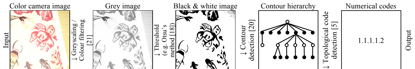
Figure 6. Image processing workflow for detecting topological markers. The marker is the flower.
