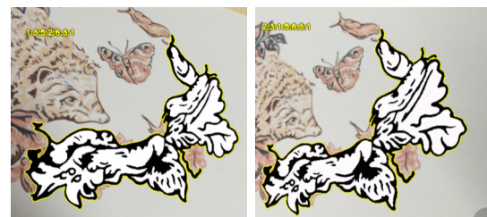
Figure 13. Scanning an auto-generated marker from different angles to yield different codes (1.3.5.2.6.3.1 on the left and 2.3.1.5.6.3.1 on the right). Uses debug mode to reveal the code.
