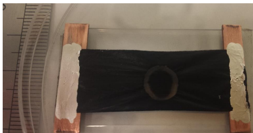
Figure S1 | As-is CNT textile made by our in-house floating catalyst CVD process is suspended from its ends above a glass slide ( top ). After illumination at one point on the surface, a transparent annulus region appears ( bottom ).
