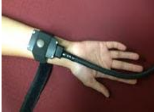
Figure 17: Peltier thermode attached to the subject's hand
