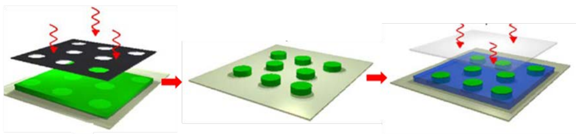
Figure 1.11. Schematic of the photopatterning process[32].
