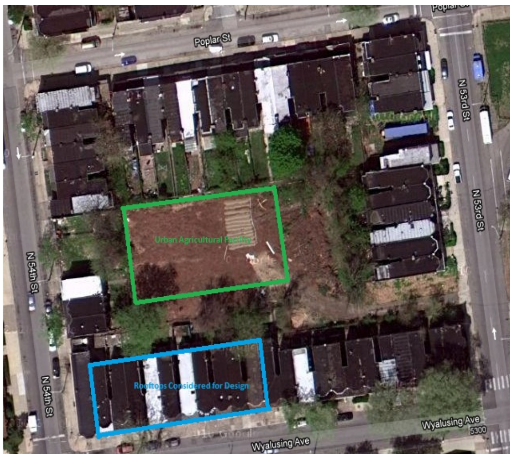
Figure 1. Google Satellite roof imagery depicting the rooftop catchments in blue and the urban agricultural facility in green (Google, 2010)
