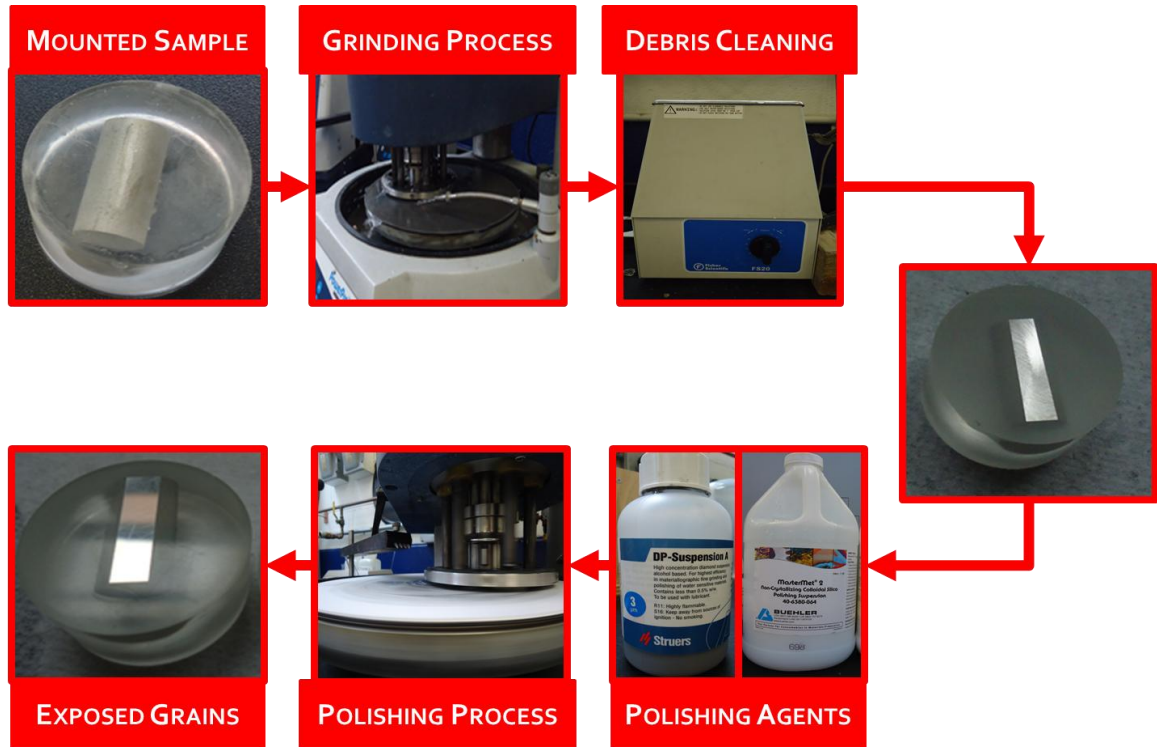
Figure 50: Mgaz31 sample preparation procedure
