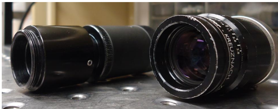
Figure 51: Left - Variable length extension tube; Right - 50 mm lenses
