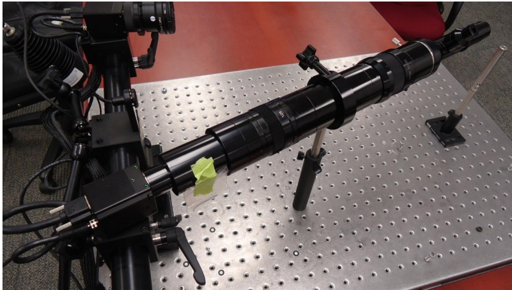
Figure 57: DIC camera augmented with the K2 long distance microscopy lens, both mounted on an optical table
