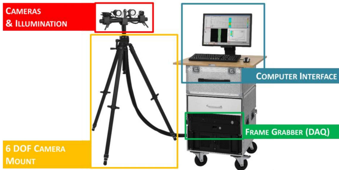
Figure 22: A typical Digital Image Correlation System
