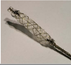
Fig. 29. 6-channel braided epidural stimulation electrode. Size of the electrode was 2cm (length) \times 0.5cm (width) \times 0.1 cm (thickness).
