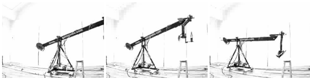
Figure 8.1: A boom fully actuated. The motion is precisely prescribed and repeatable.
