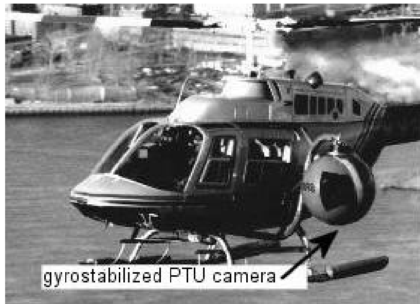
Figure 1.1: A traffic helicopter is often equipped with a camera. The pilot concentrates on safely flying the helicopter while an operator handles the camera.
