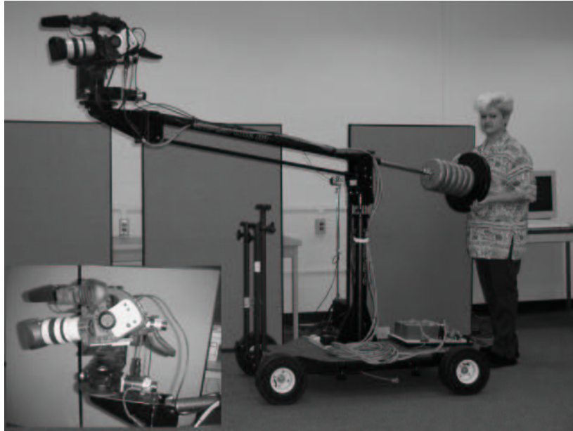
Figure 1.3: An operator can boom the arm horizontally and vertically to position the camera. The pan-tilt head (lower left inset) provides additional degrees-of-freedom.
