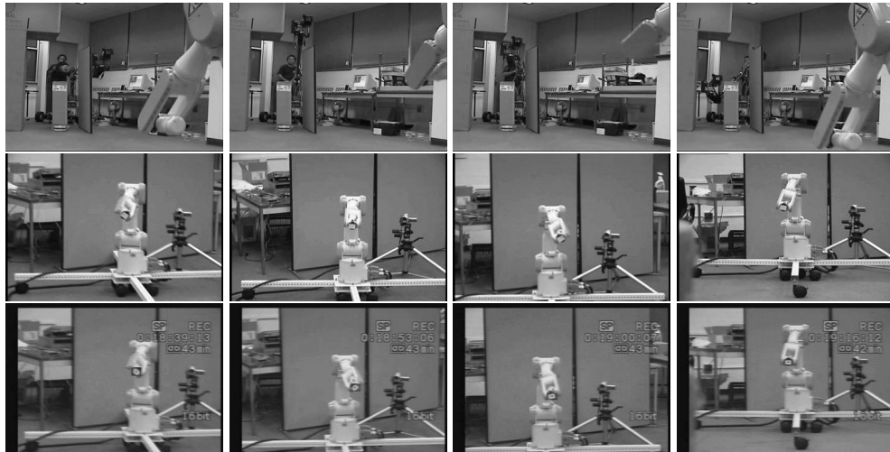
Figure 7.16: Inexperienced operator with vision system. It can be seen that target is much closer to the image center in comparison to any other experiment.
