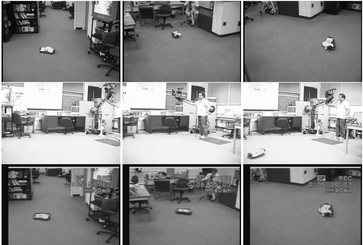
Figure 4.7: Three sequential images from videotaping the Cye robot tracking experiment using the feedforward controller. Top row: camera field-of-view shows target is tracked. Middle row: boom manually controlled. Bottom row: the working program.
