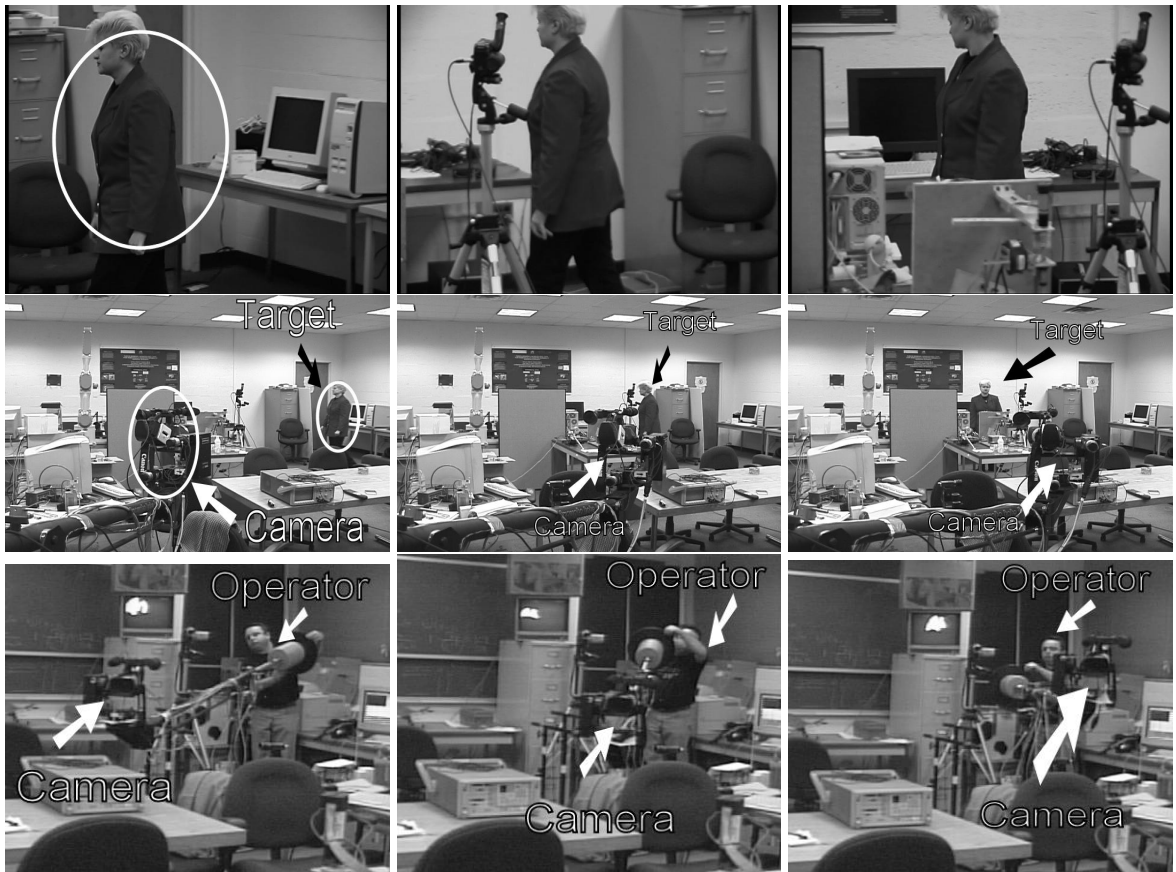
Figure 3.4: Three sequential images from videotaping the experiment. Top row: camera field-of-view shows target is tracked. Middle row: boom manually controlled. Bottom row: view from another camcorder.
