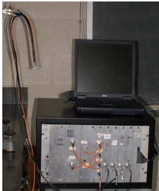
Figure 14: Photograph of frequency-domain diffuse near infrared system
