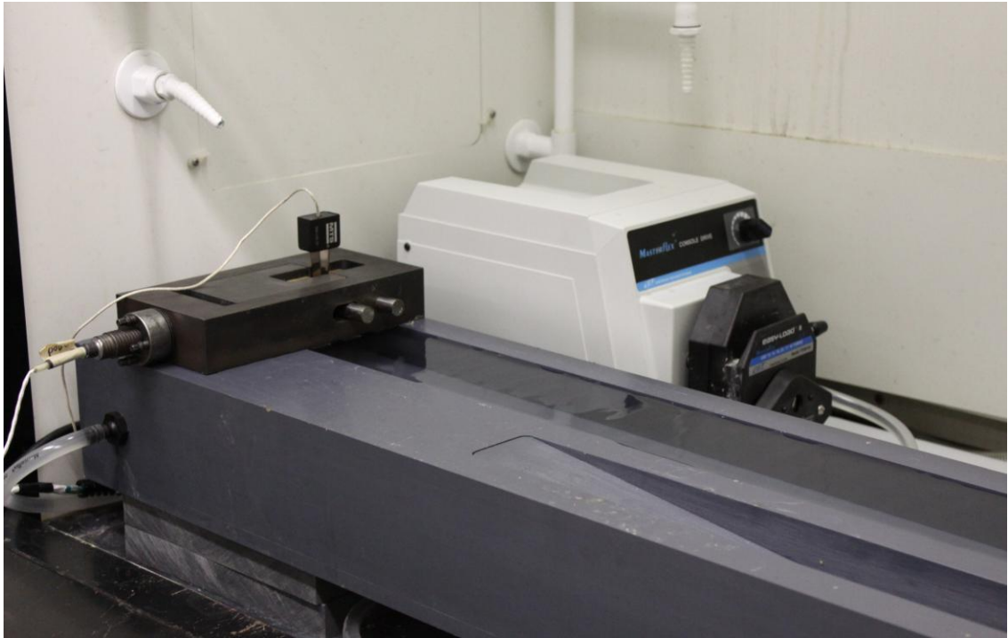
Figure 24: Hydrogen Embrittlement Test System Operating
