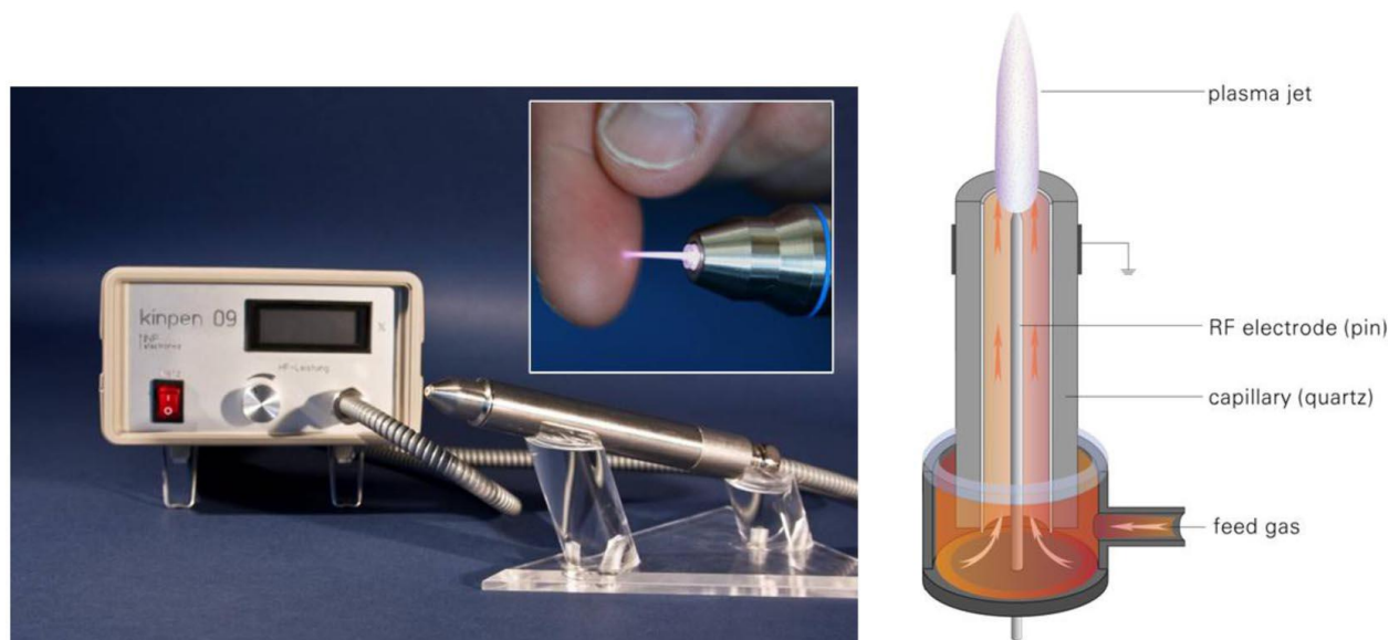
Figure 6 Atmospheric-pressure plasma jet (APPJ; INP Greifswald, Germany) for experimental biomedical applications (left: CE approved device; right: schematic set-up) [46].
