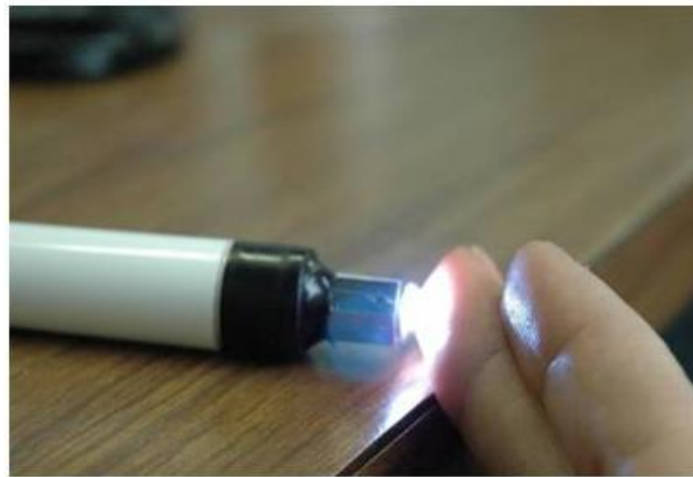
Figure 9 Pin-to-Hole spark Discharge (PHD) plasma system schematic and in operation, demonstrating that the plasma discharge is safe to the touch.
