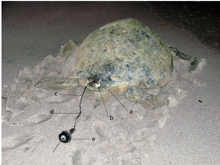
Figure 2.1: Satellite transmitter attachment to an East Pacific green turtle. a) posterior marginal scute. b) upper plastic button. c) flexible lanyard (400 lb monofilament fishing line). d) corrosive link with metallic crimps and swivel. e) Satellite transmitter (Mk 10 PAT tag, programmed for opportunistic transmissions)
