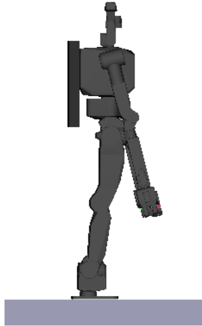
Figure 6.5: Balance failure point from simulation compared to prediction from CWS.
