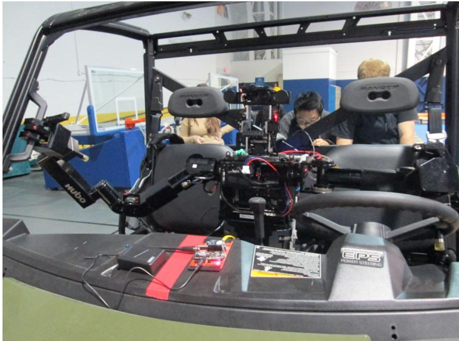
Figure 7.10: DRC-Hubo manually made to sit in a drive ready pose
