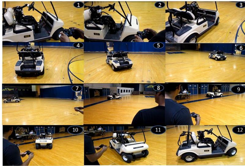
Figure 6.9: DRC-Hubo teleoperated to drive in a circular pattern
