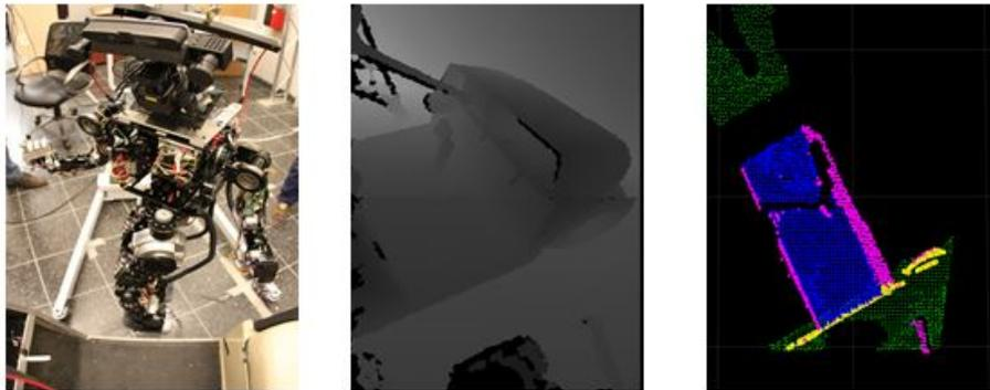
Figure 5.7: Hubo 2+ in the docking phase before performing ingress(left), Depth image from robot's point of view(center),rviz screen shot shows segmented vehicle's floor(blue) and edge(yellow) that guides the docking motion(right)
