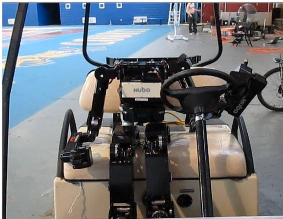
Figure 2.2: Humanoid robot DRC-Hubo seated in a driving position.
