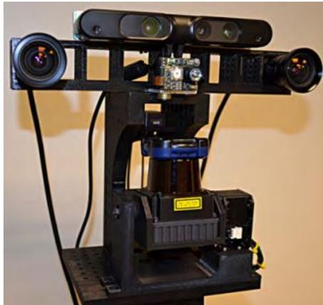
Figure 5.1: Prototype of the sensor head with Asus Xtion Pro Live and tilting Hokuyo UTM-30LX-EW, Stereo color cameras, and a PMD CamBoard nano
