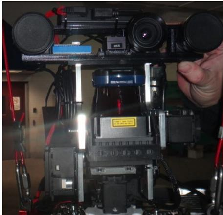
Figure 7.2: Sensor head equipped with a Hokuyo LIDAR,3 FLEA-3 CCD cameras at the top,a Microstrain IMU. The sensor head is mounted on a pan and tilt unit
