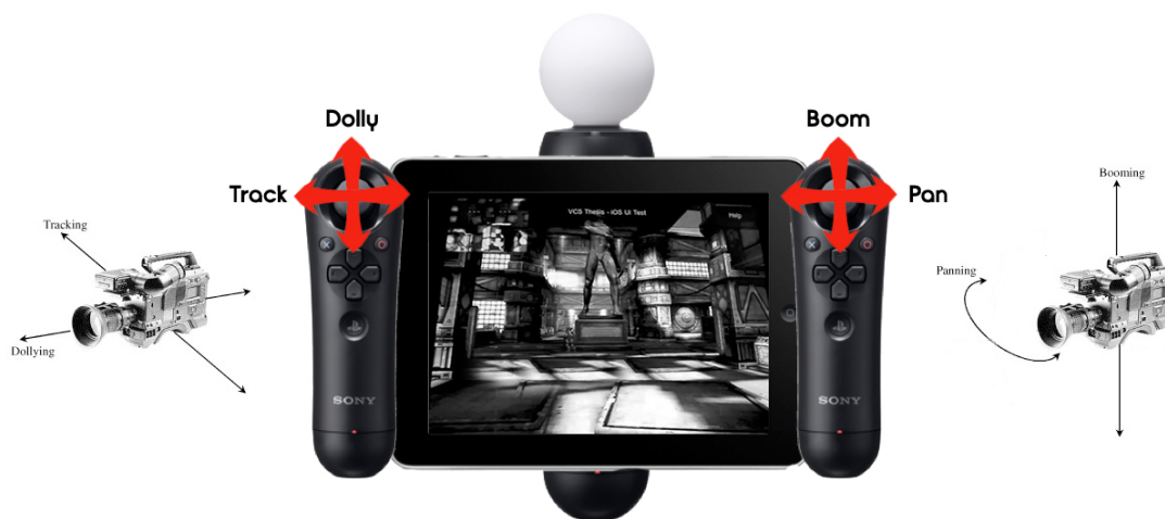
Figure 4.7: Analog Joystick Controls for the Virtual Camera: Track, Dolly, Boom, Pan
