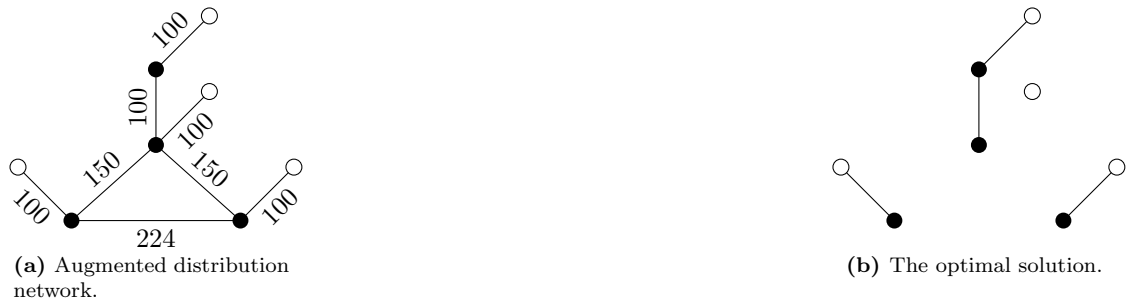
Figure 5.4: (a) gives the augmented graph corresponding to the distribution network in Figure 1.2a with a uniform depot opening cost of 100. Original vertices are \bullet and the special depot vertices are \circ . (b) is the optimal solution to the augmented network, corresponding to the solution in Figure 1.2b.
