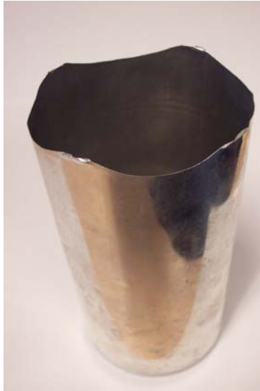
Figure 3 Earring in deep drawing of aluminum due to crystallographic texture. Compliments of Dr. Roger Doherty, Drexel University.
